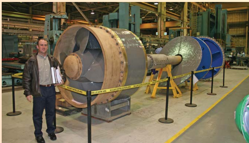
Axial view of pump internals from the suction bell (bottom) up past the diffuser to the drive coupling (top). The five AR-1 bearings are situated along the shaft.
