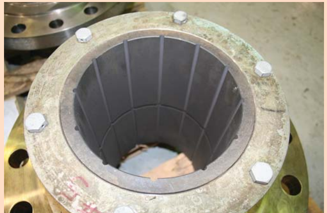
AR-1 axial fluted and pinned bearing inside flanged bearing housing.
