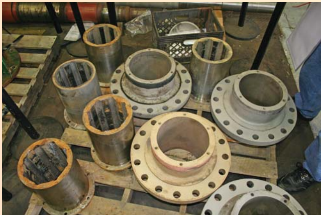
Disassembled flanged bearing housings with failed rubber cutlass bearings removed.
