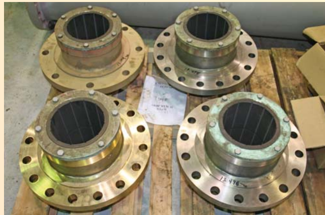
AR-1 bearings installed in flanged bearing housings.
