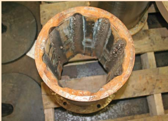
Close-up of failed rubber cutlass bearing.
